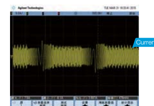
Current waveforms in vector control mode with 50Hz and full load
